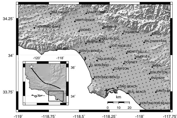
Figure 1. Scope of study area. Small triangles indicate locations where ground motion time histories are computed. Major cities are shown for reference. The inset shows the rupture trace in relation to the study area and the star represents the rupture initiation point (Parkfield).
