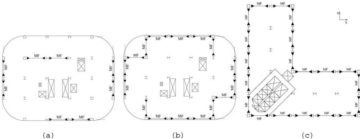
**Figure 3.** Typical floor plans are shown for the three buildings modeled: (a) Building 1, an existing 18-story building designed according to the 1982 UBC; (b) Building 2, a redesigned version of Building 1 conforming to the 1997 UBC; and (c) Building 3, a 19-story L-shaped building designed according to the 1997 UBC. Bays marked “MF” indicate moment frames.
